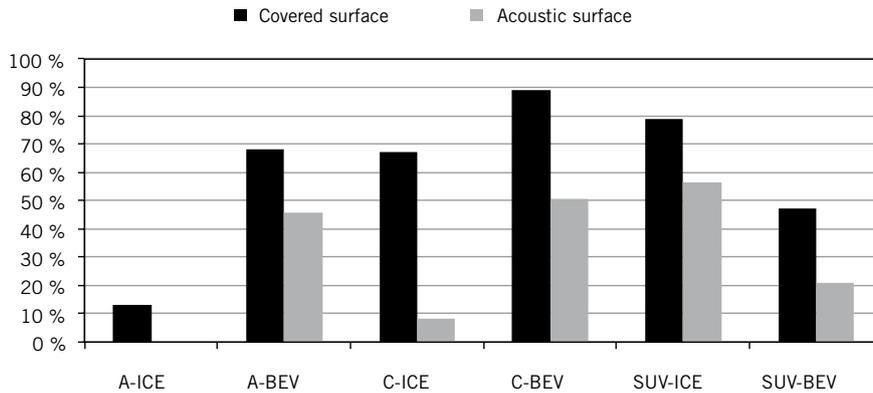
FIGURE 5 Underbody coverage rates as a percentage of the total underbody surface (© Autoneum)
