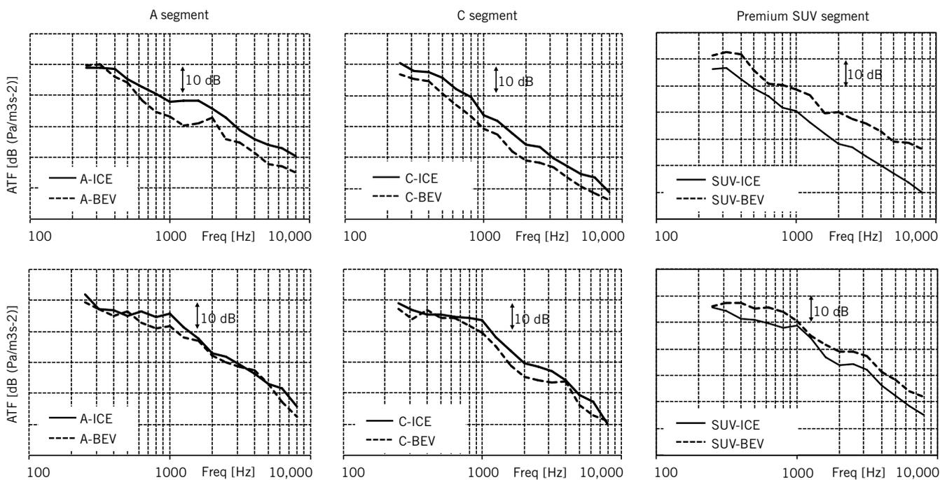
**FIGURE 4** Air-borne transfer functions (© Autoneum)
