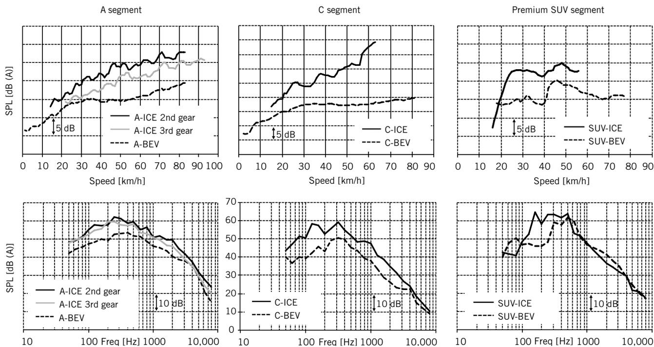
**FIGURE 2** Acceleration test results (© Autoneum)
