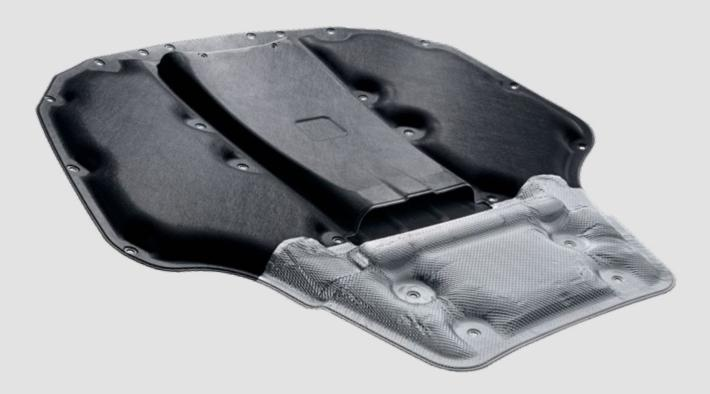
Theta-Cell is an innovative polyurethane foam material developed by Autoneum. It is used for different applications such as lightweight and multifunctional hoodliners, outer dashes, tunnel insulators and battery covers. Compared with conventional acoustic absorbers, Theta-Cell components can be used to achieve weight reductions of up to 60% as well as high thermal insulation.
