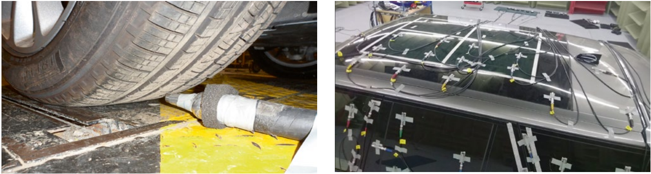
FIGURE 2 Source at the tire (left) and microphones placed on the roof panels (right) © Autoneum
