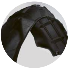
Wheelhouse outer liners
